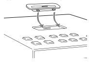
To remove the iPod Dock Adapter, pull it up with your fingernail or a flat object using the slot inside the adapter.
